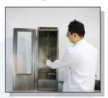
Sample holder and sample as vertically hanging in test chamber.
